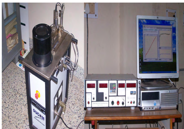
Fig. 1. Schematic setup of wear test.
